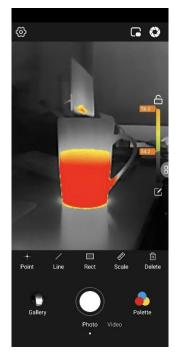
The isotherm scale can be used for palettes other than white-hot or black-hot to highlight the temperature zone requiring special attention. The selected zone is displayed in the form of a palette while others are white-hot.
