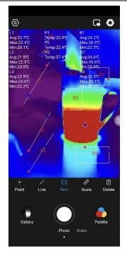
Only point-based temperature measurement supports adding or dragging measurement points. To delete a measurement point, tap the point. This is also the case for other controls.
